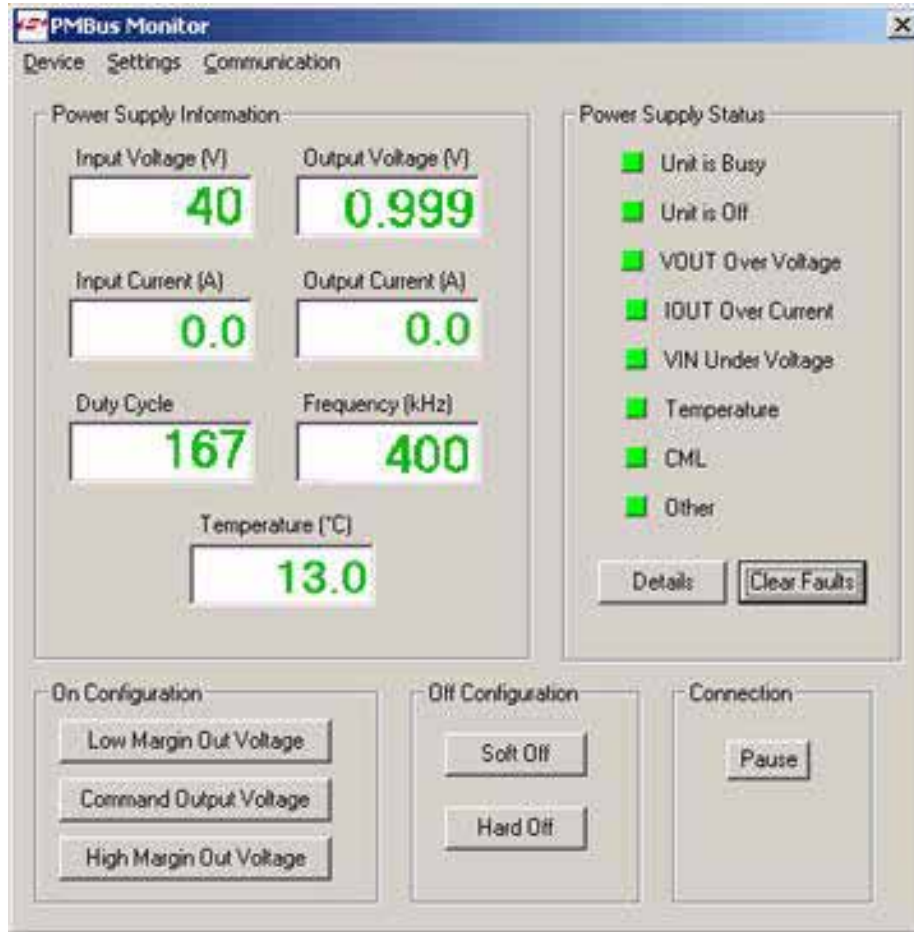
Figure 5. View of the PMBus Monitor
